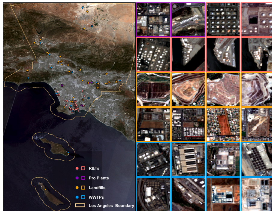
Fig. 8. Detected methane-emitting facilities in Los Angeles. (Left: Overall facility distribution; Right: Enlarged views of facility types. Background imagery: Sentinel-2 true-color composite [RGB: Bands 4/3/2]).
